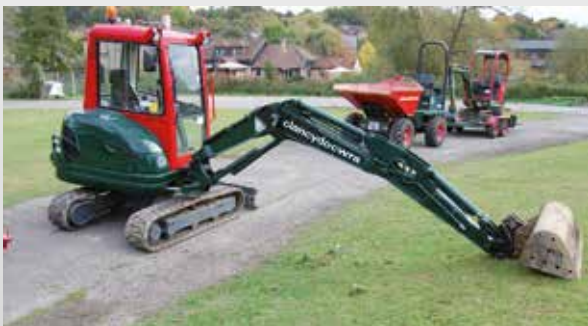
If leaving mini excavators remove from trailer, slew cab and extend boom arms. Use immobilisers and/or hydraulic locks. This makes the machine impossible to remove or lift away. Note the use of CESAR registration and corporate livery. Criminals dislike stealing this type of equipment due to expense of repainting equipment.
