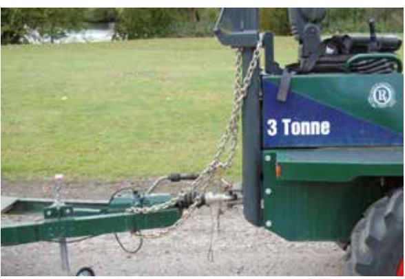
Secure trailers and equipment to each other or to road furniture. Lift all chains from ground to prevent easy attacks and purchase for cutters/bolt croppers. Invest in good quality approved chains and padlocks.
