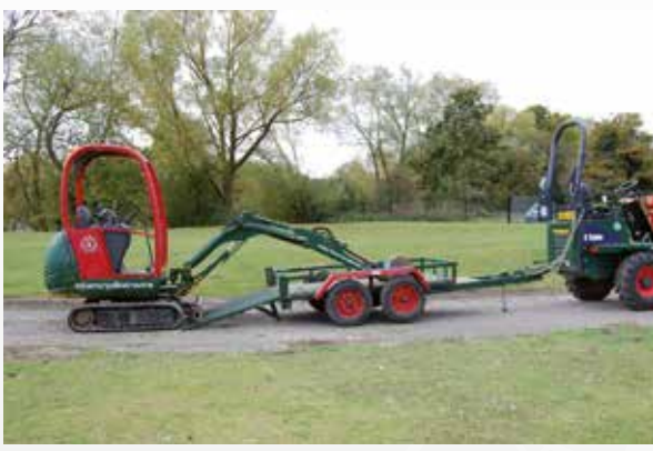
Make the thieves life harder. Equipment removed from trailer and boom arms extended and immobilisers and /or hydraulic locks set preventing ease of theft.
