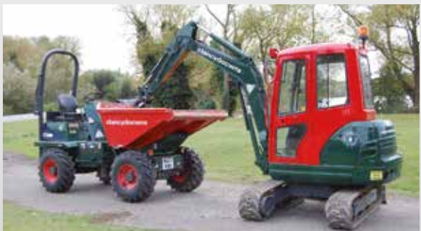
Secure equipment together preventing either being lifted or dragged away. Use immobilisers and/or hydraulic locks with chain and padlocks.
