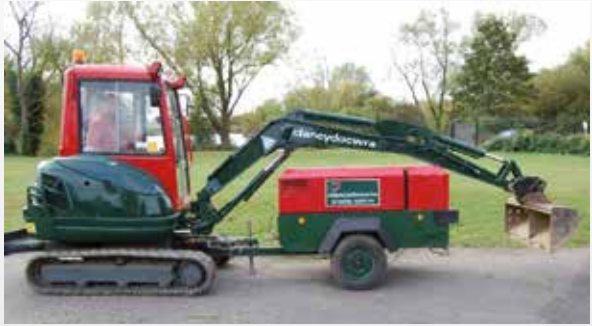
When leaving equipment overnight on sites secure compressors under boom arms of mini excavators then use immobilisers or hydraulic locks to prevent removal.
