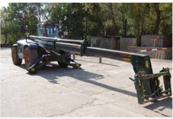
Boom arms and legs extended and immobilisers and/or hydraulic locks set. This telehandler now becomes nearly impossible to remove quickly by theft.
