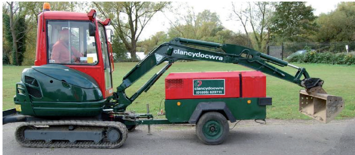
When leaving equipment overnight on sites secure compressors under boom arms of mini excavators then use immobilisers or hydraulic locks to prevent removal.
