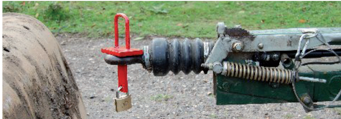
Trailer locks and tow hitch locks preventing removal.
